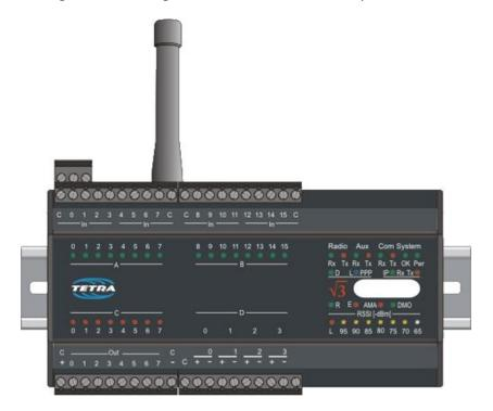
Most serial and IP based SCADA and telemetry protocols can directly be used on TETRA networks. With a polling throughput of up to 1000 Modbus RTU polling within 5 minutes on a single 25 kHz TETRA carrier, this technology can compete even against 3G. This can increase the utilisation of an existing TETRA communications system, making the investment in the technology all the more beneficial.
