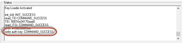
The Keyloader can now be disconnected from the TMO-100:
