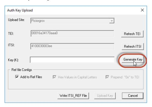
The generated key must be uploaded into the TMO-100:
